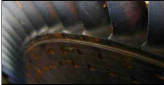
Effects of rust on static engine hardware
